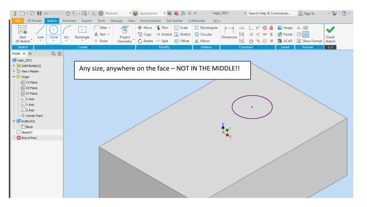
22. Select the *Dimension* tool Dimension the *Constraints* panel. Dimension the circle in three ways: (a) from the *right edge* line to the *center* of the circle, (b) from the *bottom edge* line to the *center* of the circle and (c) the diameter of the circle (select the circle). See Below – note that the below values are *random* – yours will be *different*. Hit *Escape* when done.
