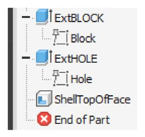
24. **Double-Click** on the *Hole* sketch. *Change the numbers* to the ones below. *Finish Sketch*. You have just *parametrically* changed the location of the hole, as well as the feature geometry – the **ExtHOLE** extrusion.
